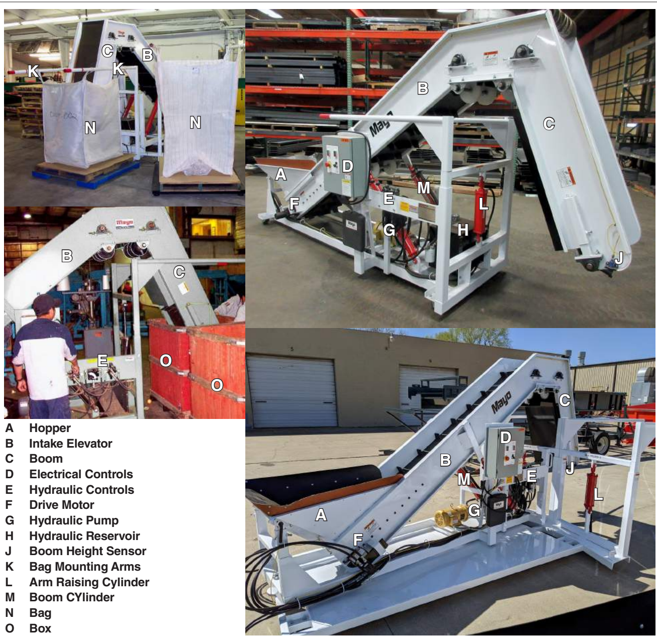
FIG. 1 MACHINE COMPONENTS
