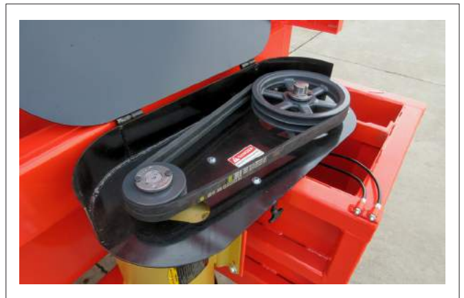
FIG. 46 PUMP DRIVE BELT
