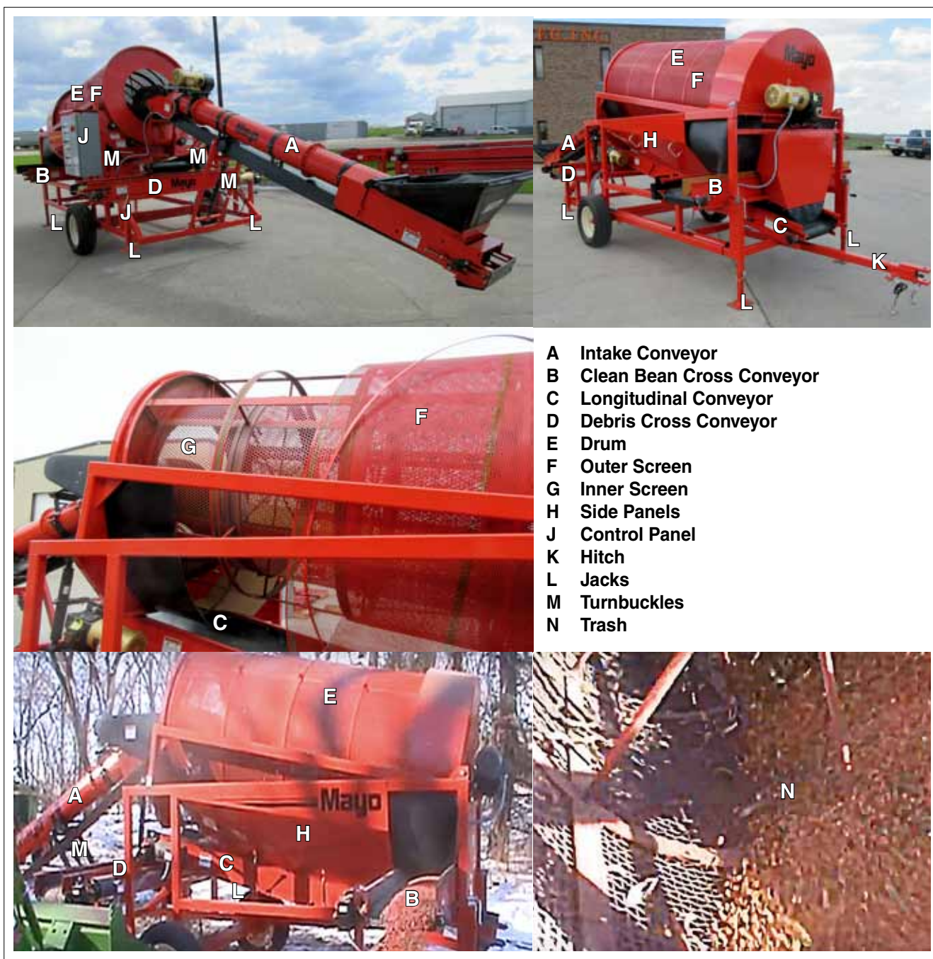
Fig. 1 MACHINE COMPONENTS
