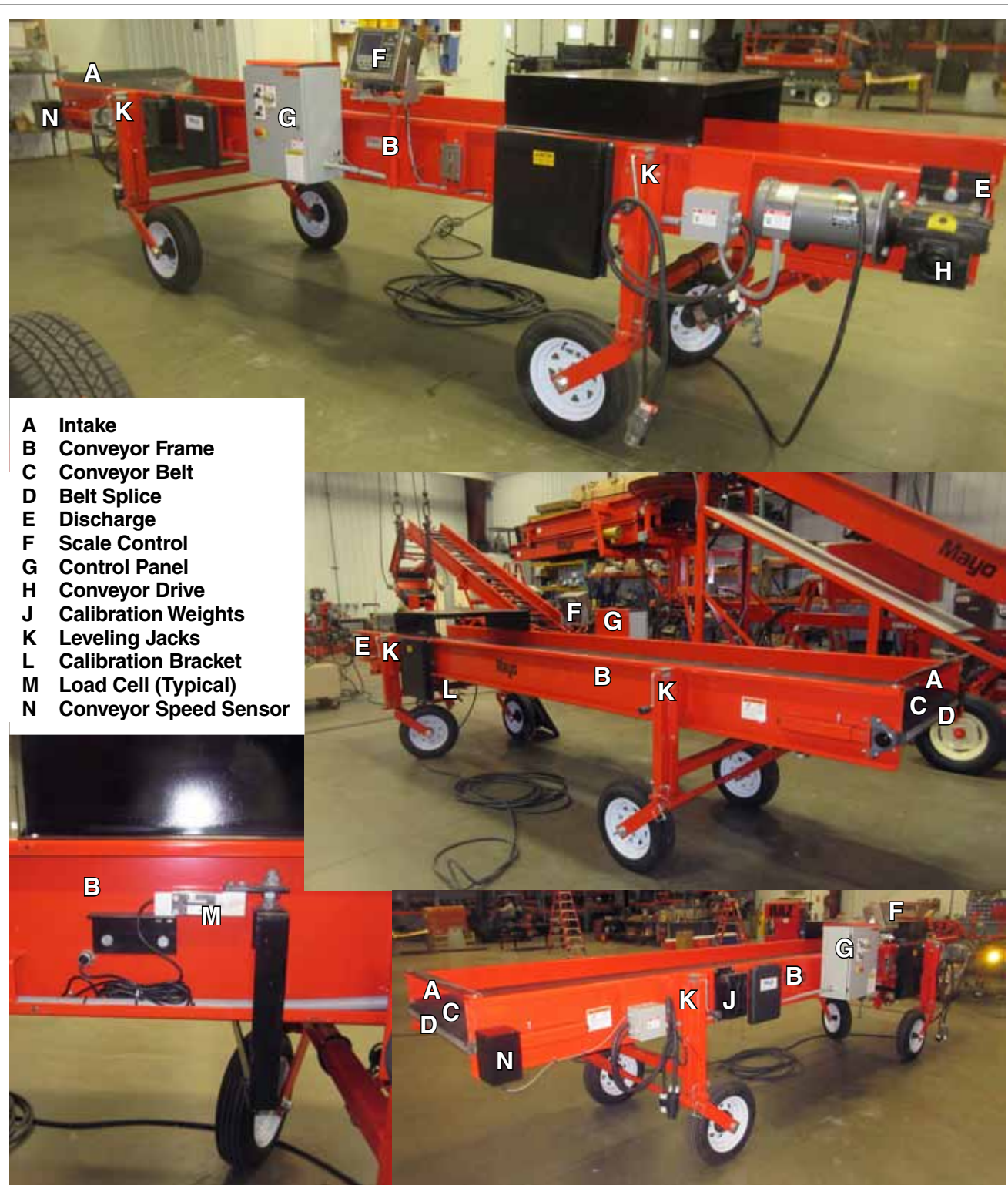
FIG. 1 MACHINE COMPONENTS
