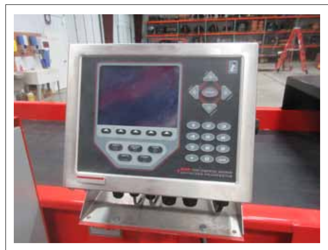
FIG. 5 WEIGH SYSTEM CONTROL PANEL
