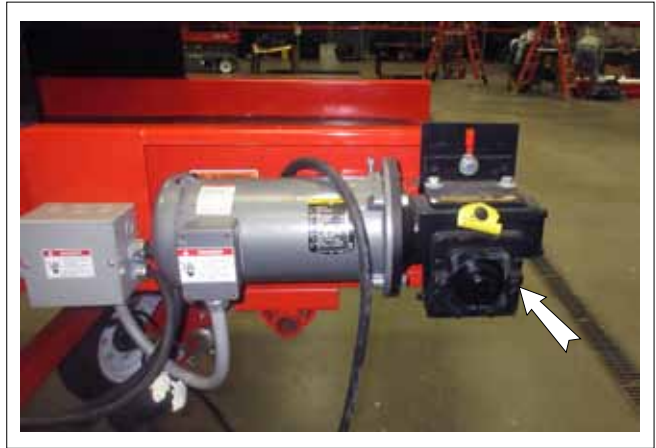
FIG. 33 LEVEL PLUG (TYPICAL)
