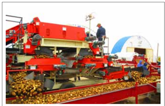
FIG. 17 CONVEYING SYSTEM (TYPICAL)
