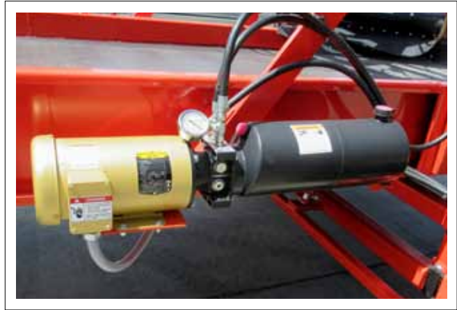
FIG. 29 HYDRAULIC SYSTEM (TYPICAL)
