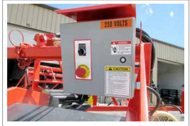
FIG. 28 CONTROL BOX (TYPICAL)
