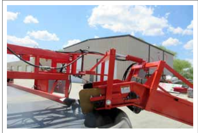
FIG. 9 ELECTRIC & HYDRAULIC LINES (TYPICAL)
