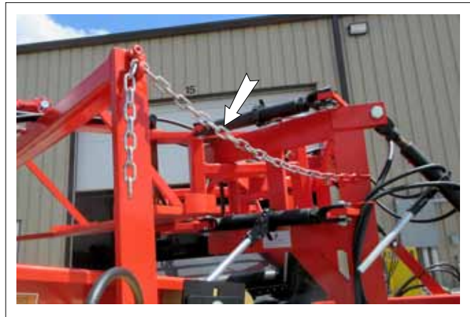
FIG. 19 SIDE SWING ANCHOR CHAIN
