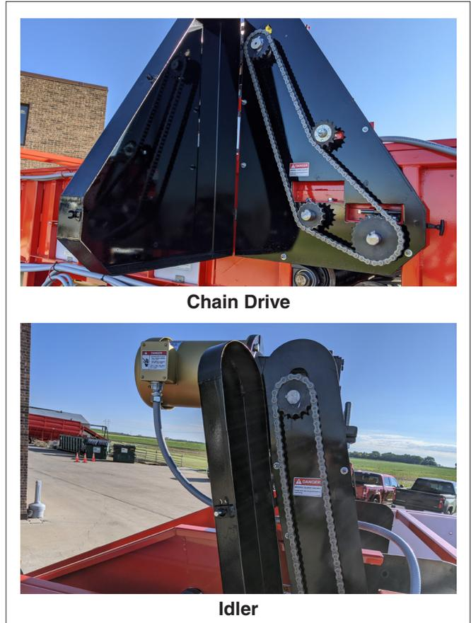
FIG. 46 TENSION ADJUSTMENT (TYPICAL)
