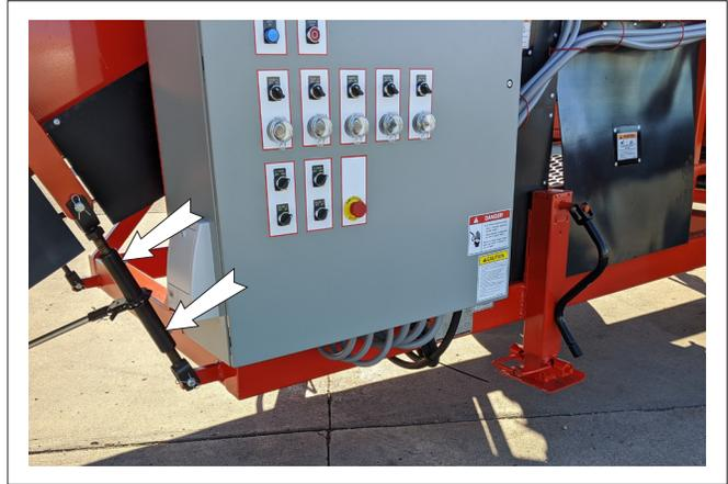
**FIG. 39 TURNBUCKLES (TYPICAL)**
