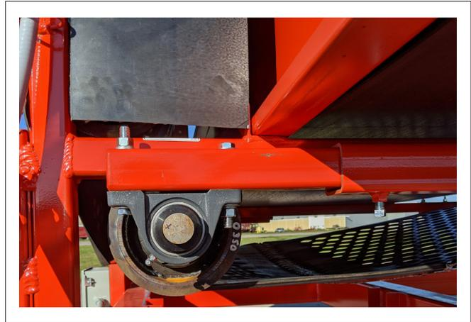
FIG. 47 TENSION ADJUSTMENT
