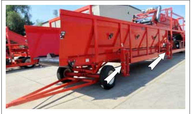
FIG. 30 JACKS/OUTRIGGERS FULLY UP
