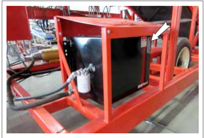
FIG. 42 HYDRAULIC OIL LEVEL SIGHT GLASS
