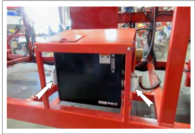
FIG. 45 HYDRAULIC SYSTEM FILTERS (TYPICAL)
