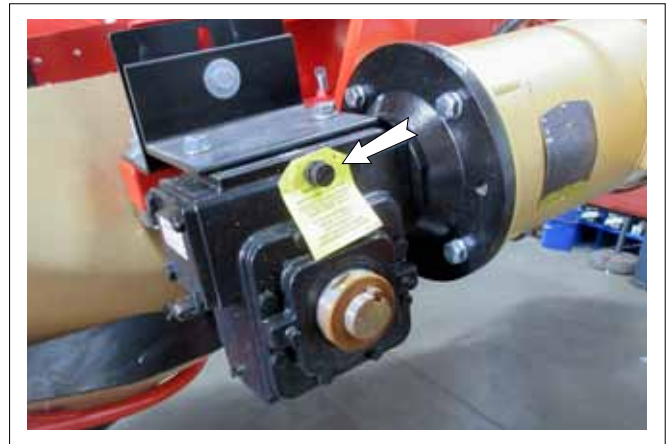
FIG. 4 GEARBOX BREATHER (TYPICAL)
