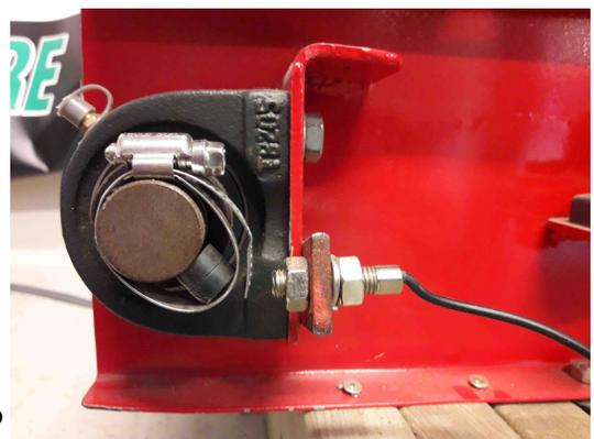
Next, prepare a sensor mounting bracket. The supplied stainless steel bracket provides a variety of
