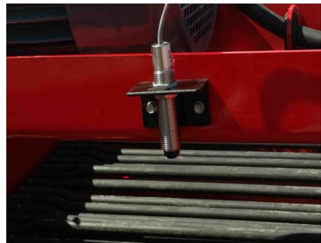
The crop temperature sensor connects to the ECU through a WA1073 cable. This cable connects to the ANALOG INPUT AIN1 terminal block: black to GND, white to AIN1, and red to +12V.
